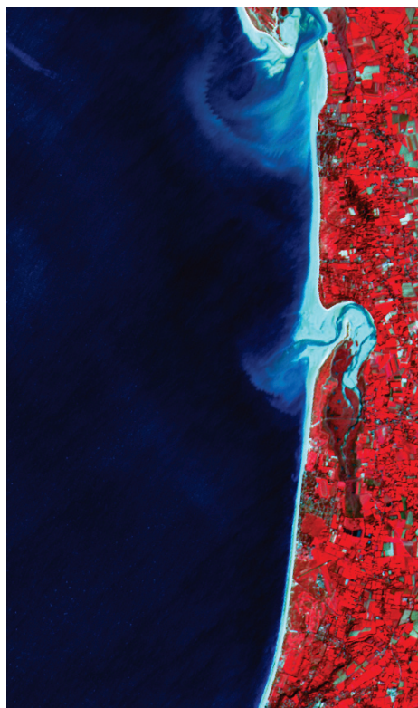
Figure 7: Composite colour (RGB) SPOT image of Lingreville (October 11, 2010 at 11:20 UTC) showing the turbid plumes exiting La Sienne and La Vanlée haven, with a Northern-Western direction.
