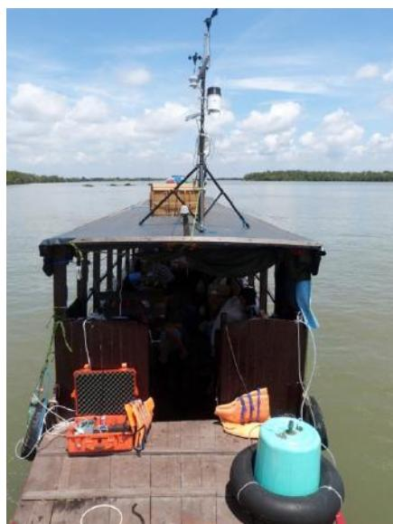
Image 1-1: Sampling boat, weather station and floating chamber used during the wet season sampling
