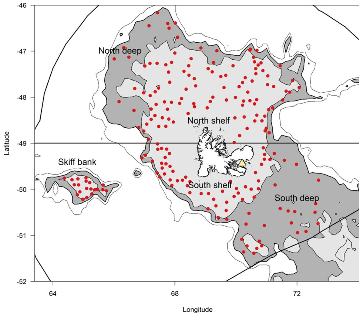
Figure 1: Map of the sampling stations of the bottom trawl surveys (POKER) in the Kerguelen Islands EEZ. The same stations were sampled over four years (2006, 2010, 2013 and 2017). Depths contours correspond to 500 m (light grey region, shallow <500 m), 1 000 m (dark grey region, 500 m to 1 000 m) and 1 500 m (not sampled). External black lines: French EEZ limits. Bathymetry source: Gebco (2014). (Δ Morbihan Bay trammel nets monitoring, 1982–1992).
