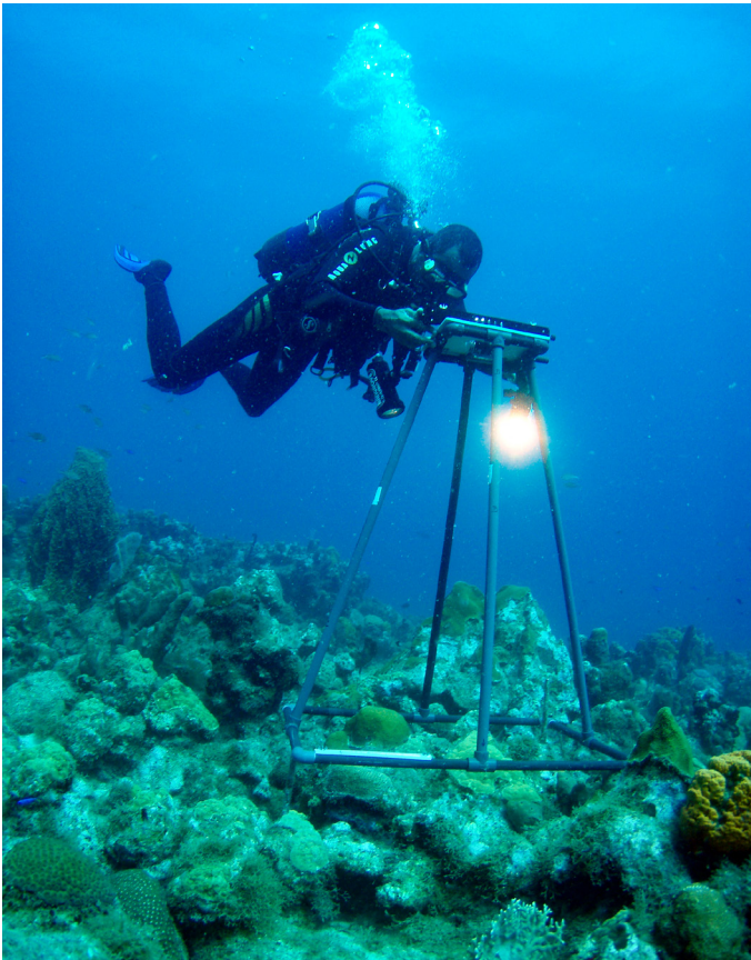
Figure 2. Photographic device used to record substrate at each quadrat. (Photo: C. Bouchon).
