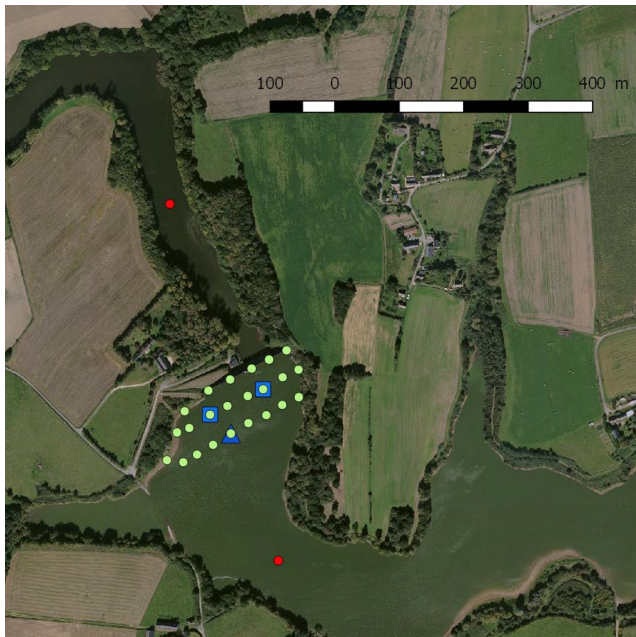
FIGURE 3 Location of the acoustic receivers with millisecond accuracy (green points) used to obtain accurate positions, and those without millisecond accuracy (red points) used to monitor the downstream or upstream movement of eels in Bois Joli Reservoir. Blue squares represent the location of the two test transmitters and blue triangle represents the position of the synchronisation transmitter (ST) and reference receiver
