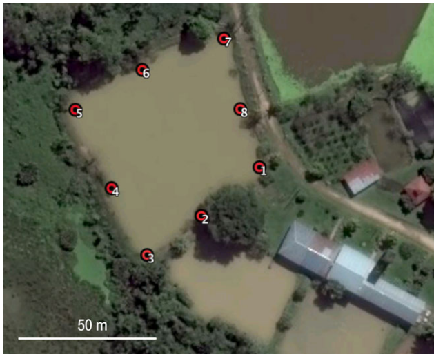
FIGURE 1 Aerial view (Google © DigitalGlobe 2016) of the zone where the experimental pond (8°24'02"S–74°38'26"W) is situated and positions of the eight hydrophones (numbered circles) forming the array inside the pond [Colour figure can be viewed at wileyonlinelibrary.com ]
