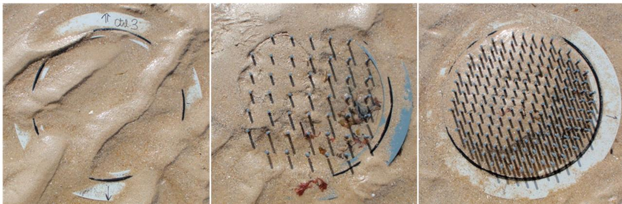
Fig. 1. Pictures of the benthic chambers 2 wk after their installation on tidal flats. From left to right: no tubes (Ctrl), low tube density (LD) and high tube density (HD) treatments
